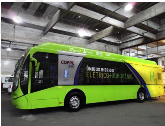
FIGURE 1.17 Example of a series hybrid battery-dominant electric hydrogen fuel cell plug-in city bus.
